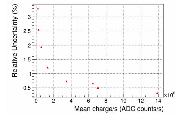
Both dosimetric observables are linear with respect to the measured dose and dose rate with independent dosimeters, and the relative uncertainty is below 5% for all dose rates.
