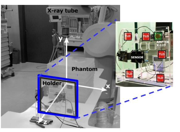
Two system observables to be used as dosimetric quantities have been defined: the number of detected photons and the mean charge per second (i.e. the sum of the reconstructed photon signals per second over a frame).
