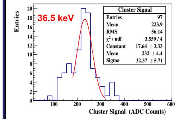
• The sensor response to the X-ray radiation has calibrated monochromatic been using (fluorescence) quasi-monochromatic or (transmission) photon beams.
